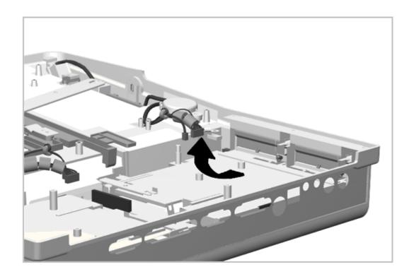
Figure 6-20. Removing the MultiBay Assembly
